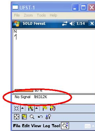
Example of GPS unit without an adequate lock on satellites. No cross-hairs nor GPS precision information.
